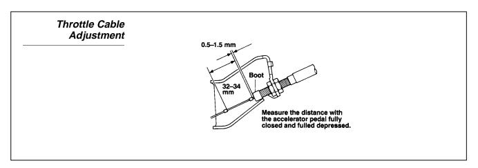
The illustration below represents yet another adjustment type. The rubber boot has a shallow extension when compared to the first one discussed earlier. The procedure differs in that the throttle is left in the fully closed position when the distance is measured from the front of the boot to the front of the stopper.
