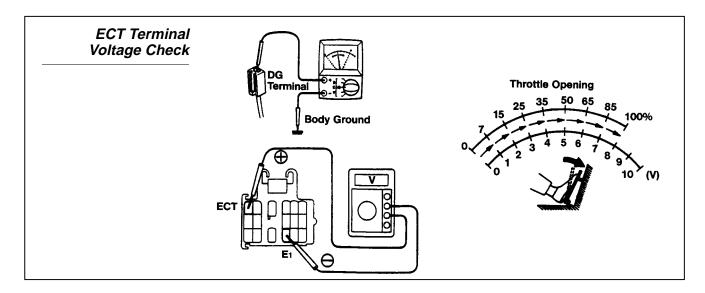
The voltage chart above provides a voltage value for the corresponding throttle opening. This can be used to establish accelerator position for a given throttle opening.
