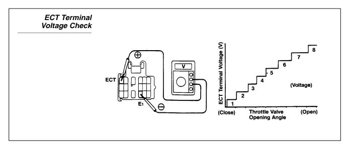
The ECT terminal can be designated as TT or Tl depending on the vehicle model. The position in the diagnostic check connector remains the same. The voltage will increase in one volt increments from 1 to 8 volts as the throttle is slowly opened. To verify the brake signal, apply the brake pedal while the throttle is wide open. The voltage displayed on the voltmeter screen will go to zero.
